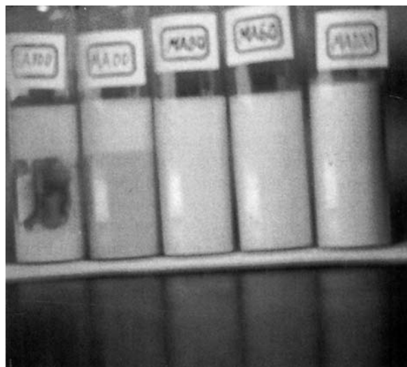
Figure 1 Monomer emulsions after 10 days. Samples (from left to right): EA100, MA00, MA30, MA60, and MA100.
